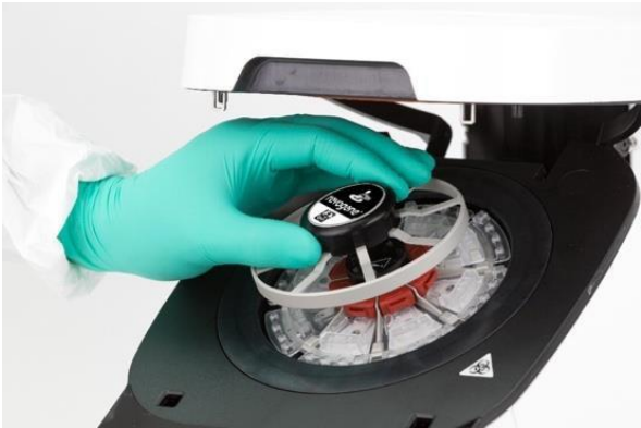
Figure 9. Placing Retention Ring
