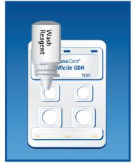
5. Hold Wash Reagent vertically and add 3 drops to each reaction (upper) port.
