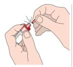
Hold the vial vertically and gently tap on benchtop. Break the tip from vial using absorbent paper.
