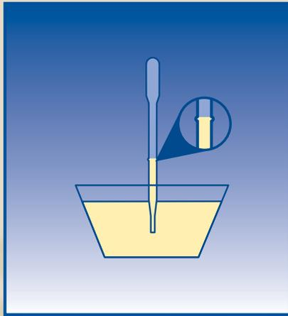
1. Squeeze the bulb of the pipette and insert the barrel into the patient sample. Release the bulb and draw up enough sample to fill the barrel to the line indicated on the pipette. Do not overfill.
